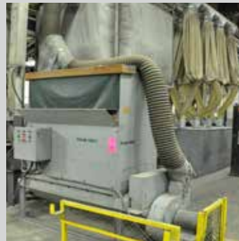
Styrofoam Reclamation System
