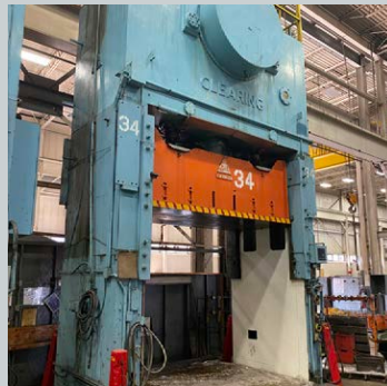
300 Ton Clearing Model S4-300-124, SSDC with Rolling Bolster
