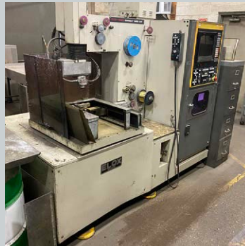
Elox Series P Wire Cut with Fanuc CNC EDM
