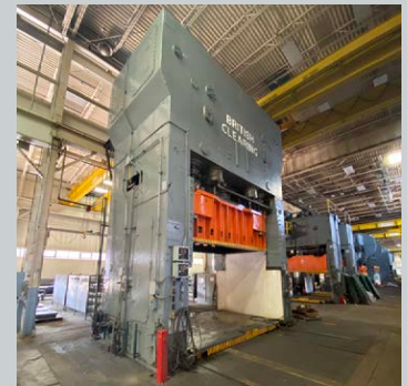
1500 Ton Clearing Model TF4-1500-180-96, Double Action, Rolling Bolster
