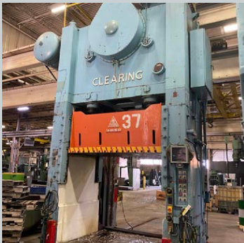
400 Ton Clearing Model S4-400-96-60 SSDC, with Rolling Bolster
