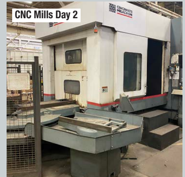
Cincinnati Magnum 5 Axis CNC Horizontal Machining Center
