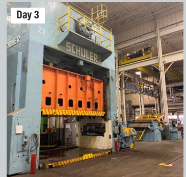
1100 Ton Schuler SSSC, 199" x 100" Rolling Bolster, with 72" x 40,000 lbs. Feed Line
