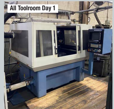
Anca Model TG-7 5 Axis CNC Tool & Cutter Grinder (2016)
