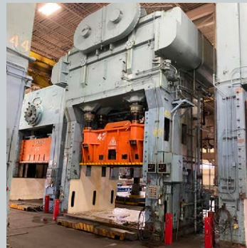
800/600,1400 Ton Clearing Model DF4-800-177, Double Action Toggle, Rolling Bolster
