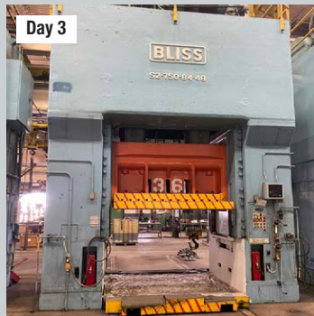
750 Ton Bliss Model S2-750. SSSC, 84" x 48" Bed, Rolling Bolster
