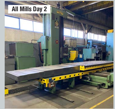
6" Model 70 A-D5-T, 128" Table Type CNC Horizontal Boring Mill
