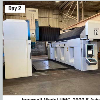
Ingersoll Model HMC-2500 5 Axis CNC Bridge Type High Speed Vertical Machining Center
