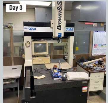
Brown & Sharpe Micro ExCell #7/10/5 Black Granite CMM with Renishaw Probe
