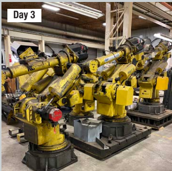
Multiple GMF Robotic Arms Model S420, 6 Axis, Material Handling Robots
