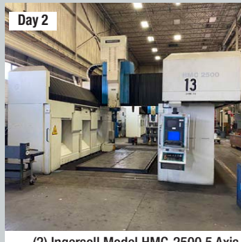
(2) Ingersoll Model HMC-2500 5 Axis CNC Bridge Type High Speed Vertical Machining Center. Die Finisher
