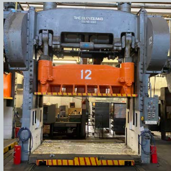
300 Ton Cleveland SSDC, 4 Point 68" x 132" Rolling Bolster
