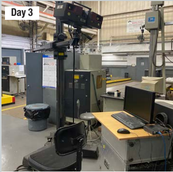
Gom Model Atos-11-Triple Scan 3-D Scanner Measuring System (2014)
