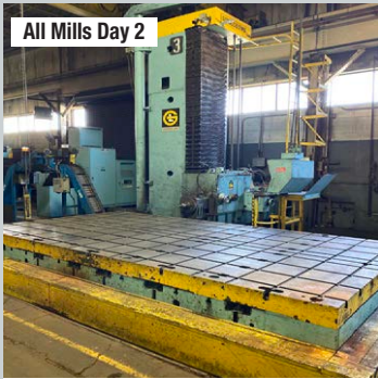
6" G & L Model G60F CNC Horizontal Floor Type Boring Mill
