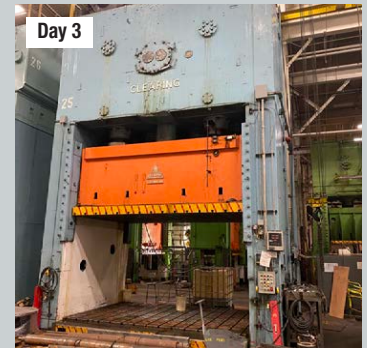
2000 Ton Clearing F4-2000-180, SSDC Press, 180" Bed Area
