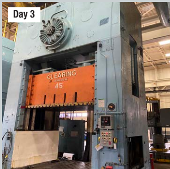
800 Ton Clearing Model S4-800-120-72, SSSC, Rolling Bolster
