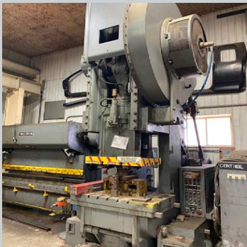
150 Ton USI Clearing OBI Punch Press, 11" Stroke, 50 x 30" Bed Area
