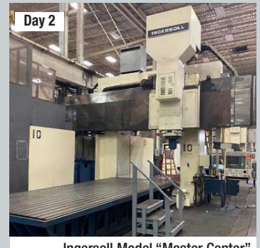
Ingersoll Model "Master Center" 5 Axis CNC 236" Table Vertical Machining Center (2) avail.
