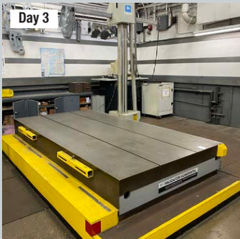
Brown & Sharpe Validator Side Mount Cantilever Arm CMM Renshaw Probe CMM
