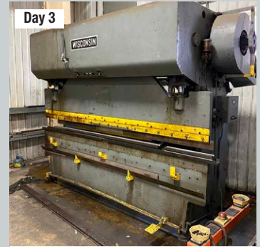
65 Ton Wisconsin 10' Mechanical Press Brake
