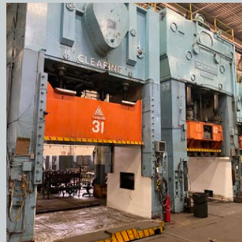
350 Ton Clearing Model F4-350-124, SSDC with Rolling Bolster
