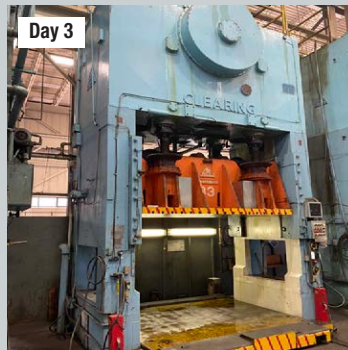
400 Ton Clearing Model F4-400-108" SSSC, Bed Area, Rolling Bolster
