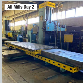
6" G & L Table Type CNC 190" Horizontal Boring Mill
