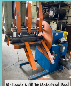
Air Feeds 6,000# Motorized Reel
