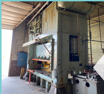
300 TON VERSON S2-300-132T TRY-OUT PRESS, 132" BED
