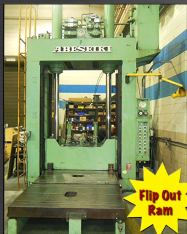
100 Ton ABESEIKI CDS-200TS Hydraulic Down Acting 4-Post Spotting Press
